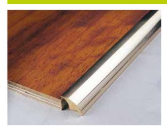
VARIOTEC DC profiles' innovative design elegantly rotates and adapts to match different floor elevations. By simply rotating its shape, this profile can adapt to floor thicknesses ranging from 9/32" to 17/32" (7 to 14mm). Use our adhesive for on-site installation.
