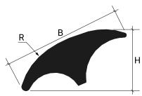
Aluminum - Brass R = 9/16" - 15 mm H for thicknesses from 7 to 14 mm - 9/32" to 17/32"
